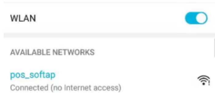
Fig. 1: The browser connects to the ESP AP
