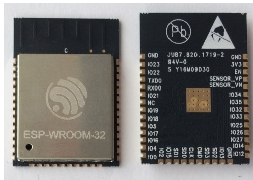
Fig. 1: ESP-WROOM-32 module (front and back)
