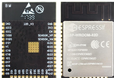
Fig. 2: ESP-WROOM-32D module (back and front)
