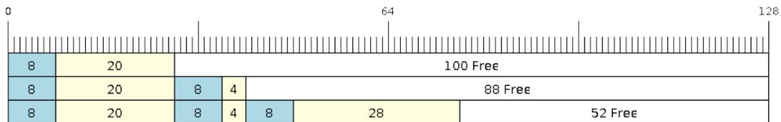
Fig. 26: Sending items to no-split/allow-split ring buffers
