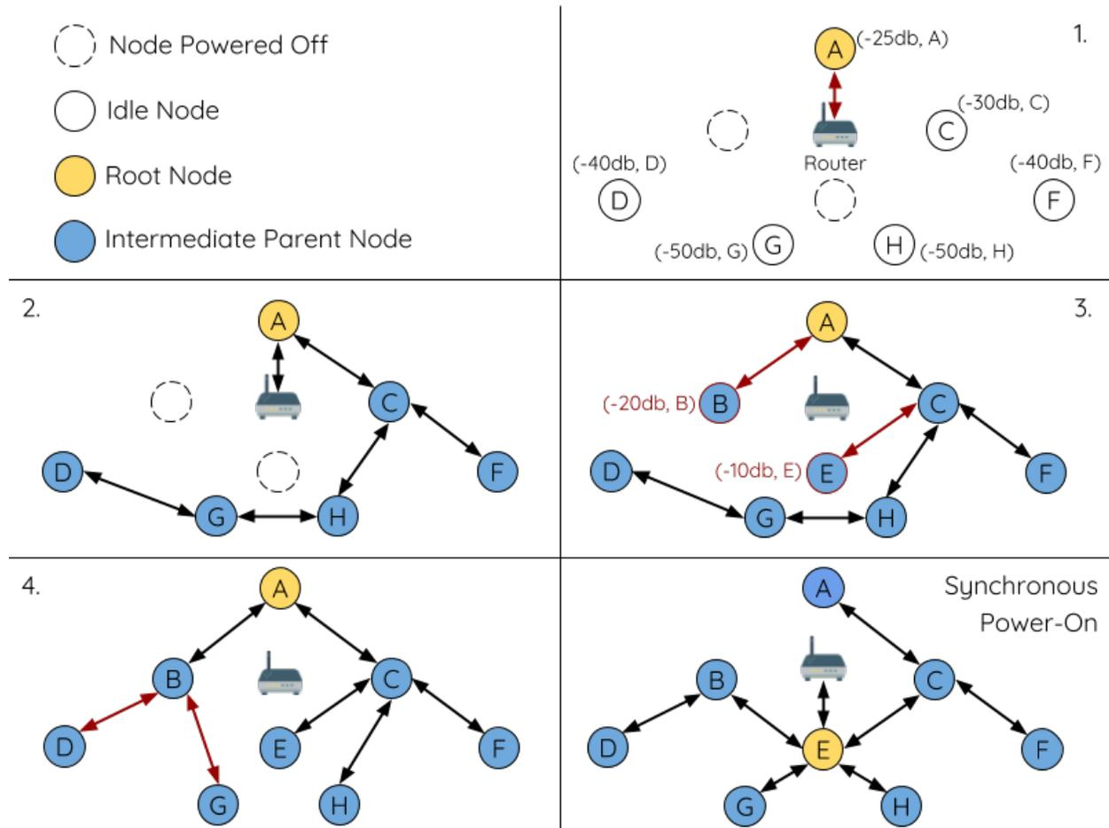
Fig. 53: Network Building with Asynchronous Power On Example
