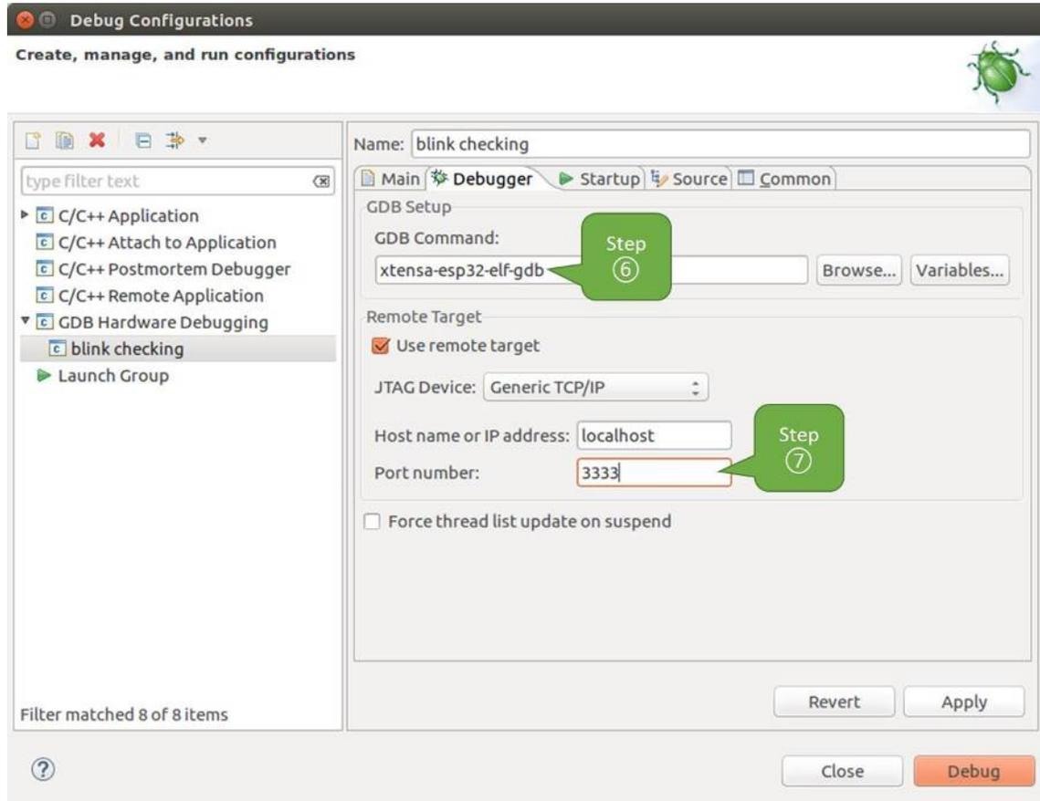
Fig. 8: Configuration of GDB Hardware Debugging - Debugger tab
