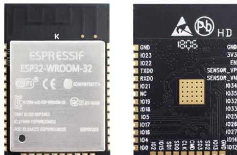
Fig. 1: ESP32-WROOM-32 module (front and back)
