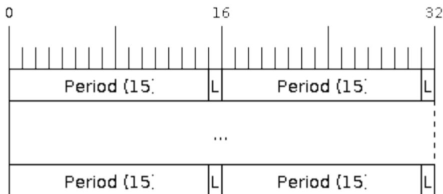
Fig. 21: Structure of RMT items (L - signal level)
