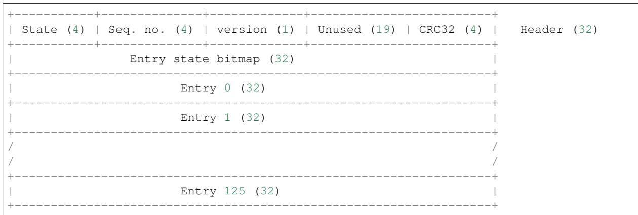
Page header and entry state bitmap are always written to flash unencrypted. Entries are encrypted if flash encryption feature of the ESP32 is used.
