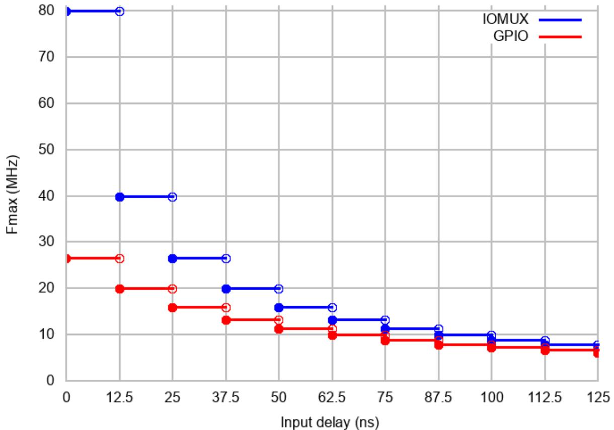
Corresponding frequency limit for different devices with different *input delay* are shown in the following table:
