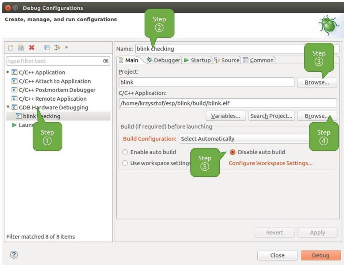
Fig. 7: Configuration of GDB Hardware Debugging - Main tab
