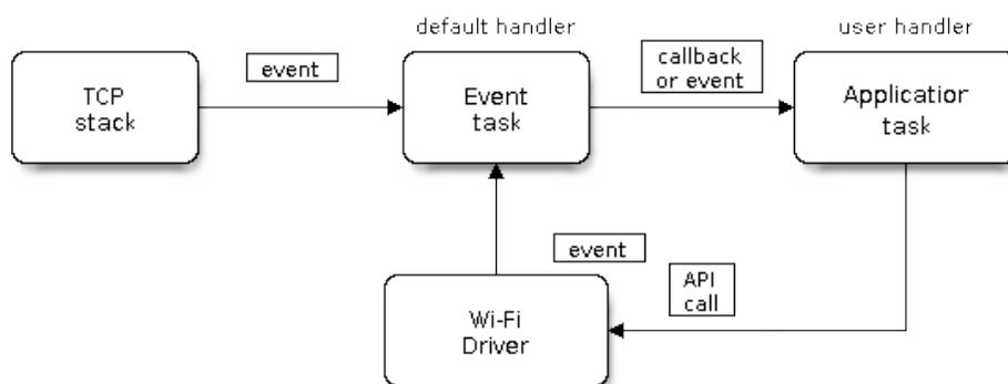
Fig. 24: Wi-Fi Programming Model
