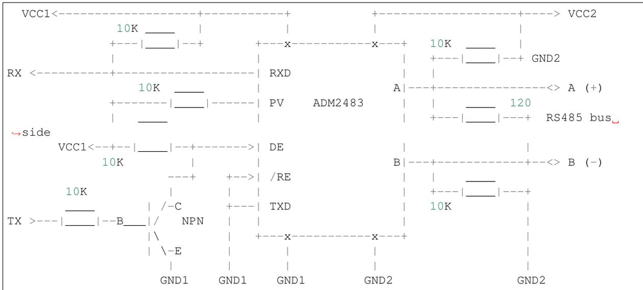
This galvanic isolated circuit does not require RTS pin control by software application or driver because it controls transceiver direction automatically. However it requires removing null bytes during transmission by setting UART\_RS485\_CONF\_REG.UART\_RS485RXBY\_TX\_EN = 1, UART\_RS485\_CONF\_REG.UART\_RS485TX\_RX\_EN = 0. This variant can work in any RS485 UART mode or even in UART\_MODE\_UART.
