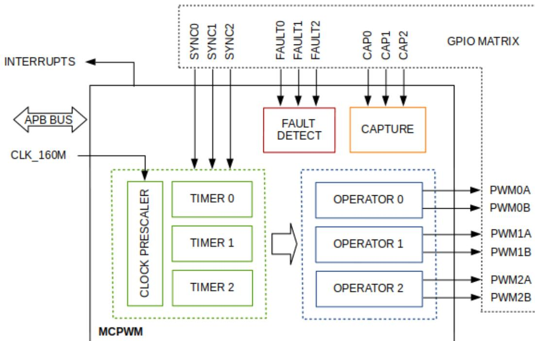
Fig. 16: MCPWM Block Diagram
