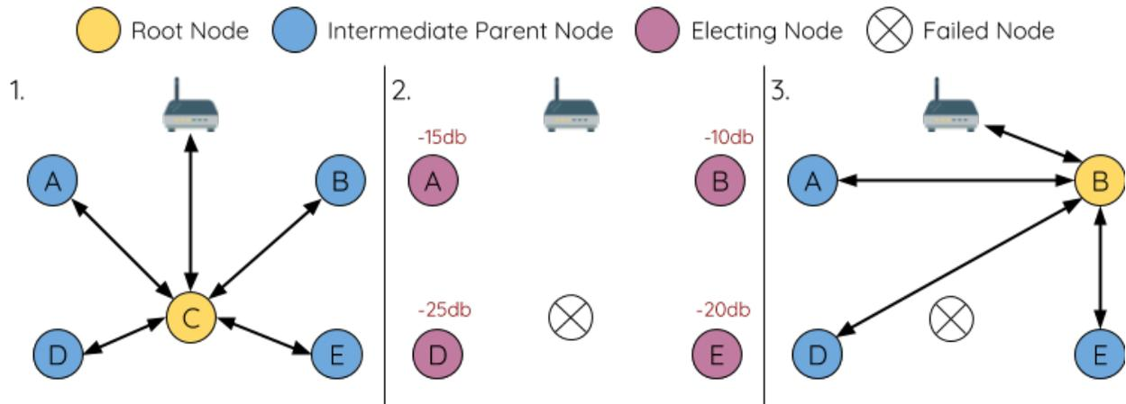
Fig. 54: Self Healing From Root Node Failure
