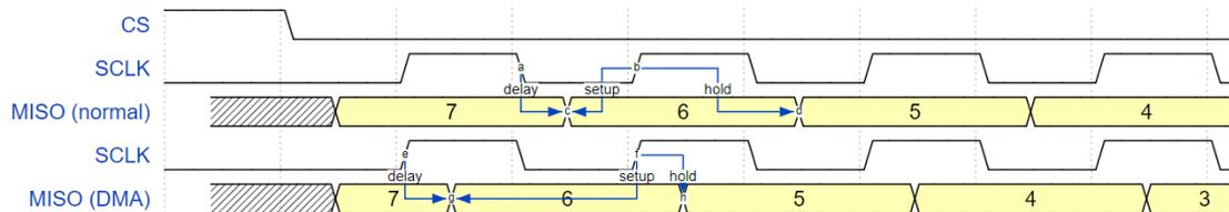
The hold time after the latch edge is 68.75ns (when GPIO matrix is bypassed), no longer half a SPI clock. The master should sample immediately at the latch edge, or communicate in mode 1/3. Or just initial the spi slave without DMA.
