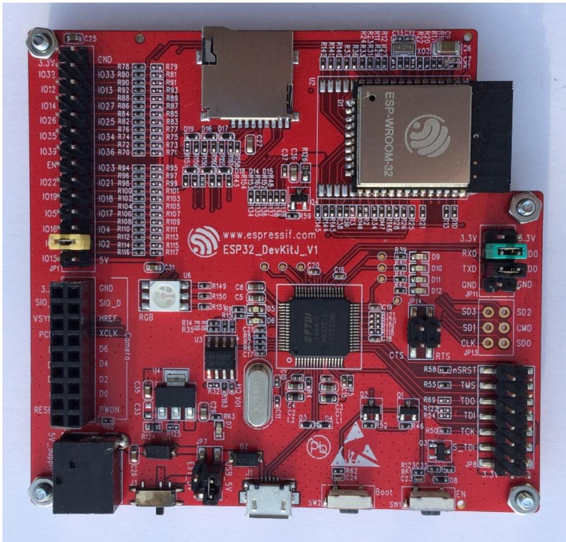
Fig. 14: ESP-WROVER-KIT V1 / ESP32 DevKitJ V1 board
