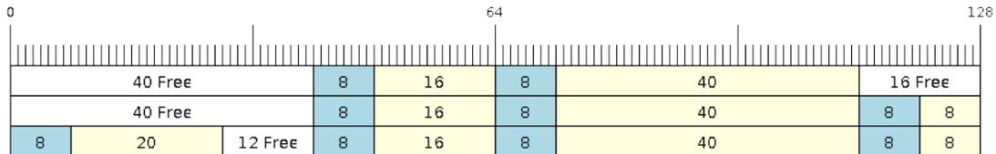
Fig. 29: Wrap around in allow-split buffers
