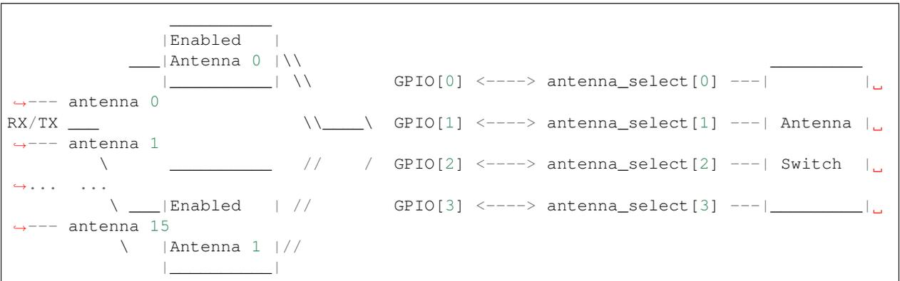
ESP32 supports up to sixteen antennas through external antenna switch. The antenna switch can be controlled by up to four address pins - `antenna_select[0:3]`. Different input value of `antenna_select[0:3]` means selecting different antenna. E.g. the value '0b1011' means the antenna 11 is selected. The default value of `antenna_select[3:0]` is '0b0000', it means the antenna 0 is selected by default.
