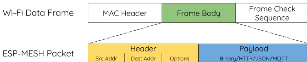
Fig. 57: ESP-MESH Packet
