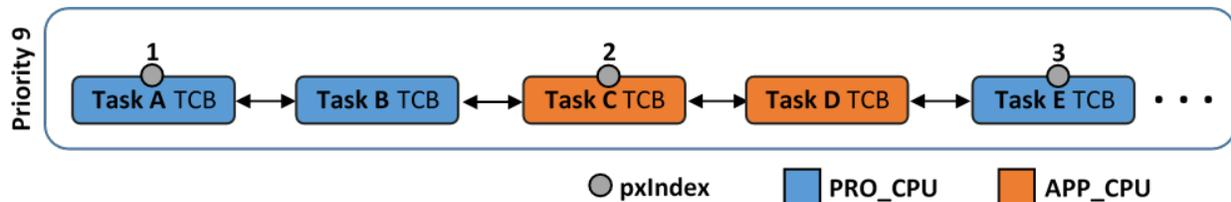
Fig. 4: Illustration of pxIndex behavior in ESP-IDF FreeRTOS
