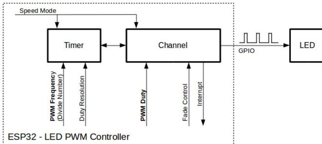
Fig. 14: Key Settings of LED PWM Controller's API
