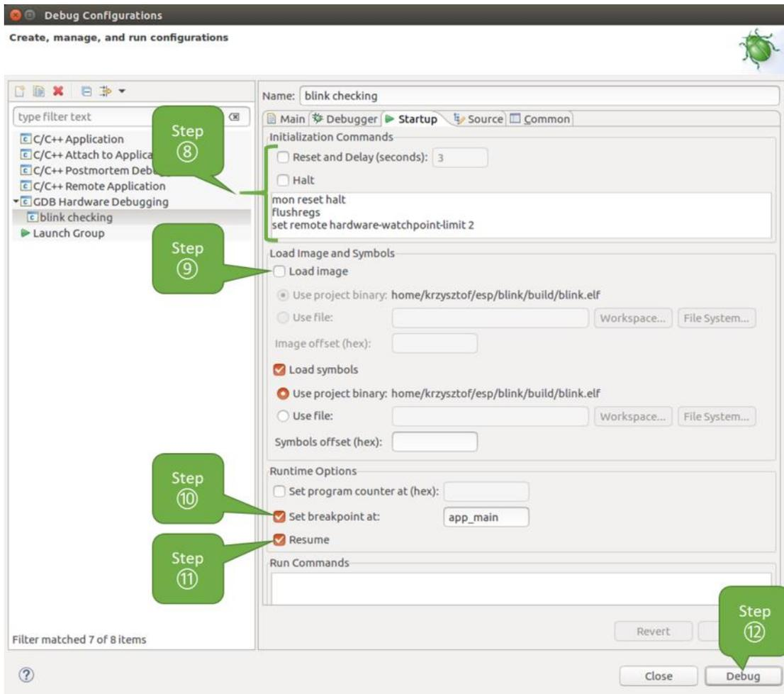
Fig. 9: Configuration of GDB Hardware Debugging - Startup tab
