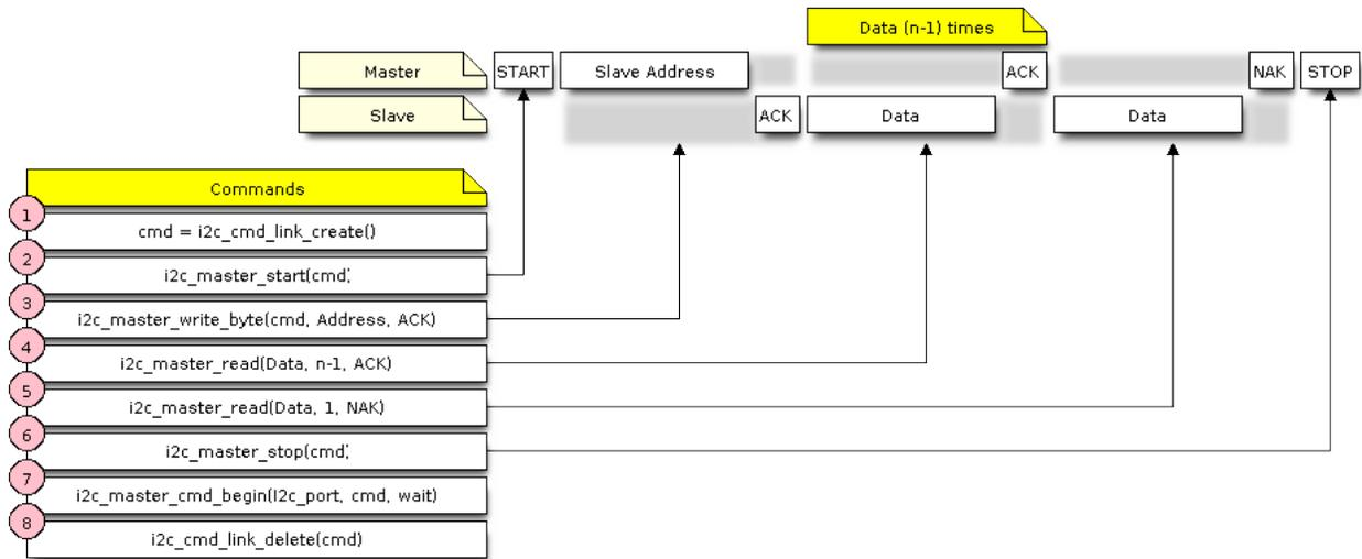
Fig. 13: I2C command link - master read example
