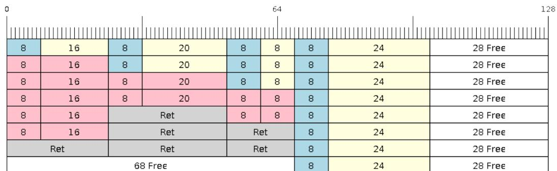
Fig. 31: Retrieving/Returning items in no-split/allow-split ring buffers
