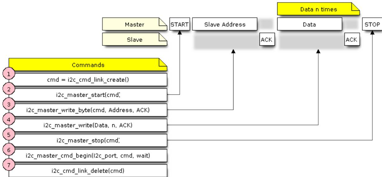
Fig. 12: I2C command link - master write example
