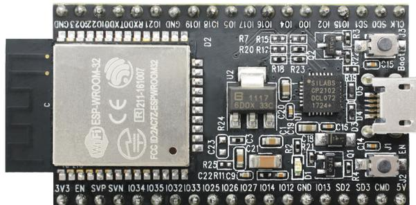
Fig. 11: ESP32 Core Board V2 / ESP32 DevKitC board
