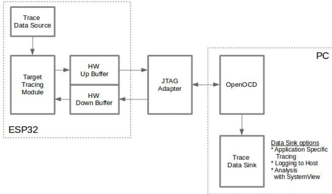
Fig. 23: Tracing Components when Working Over JTAG
