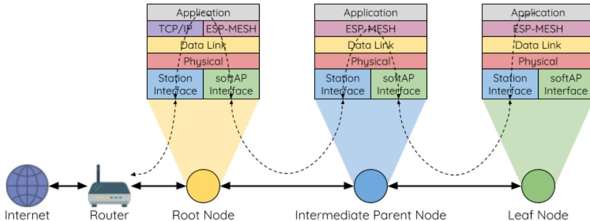
Fig. 58: ESP-MESH Bidirectional Data Stream
