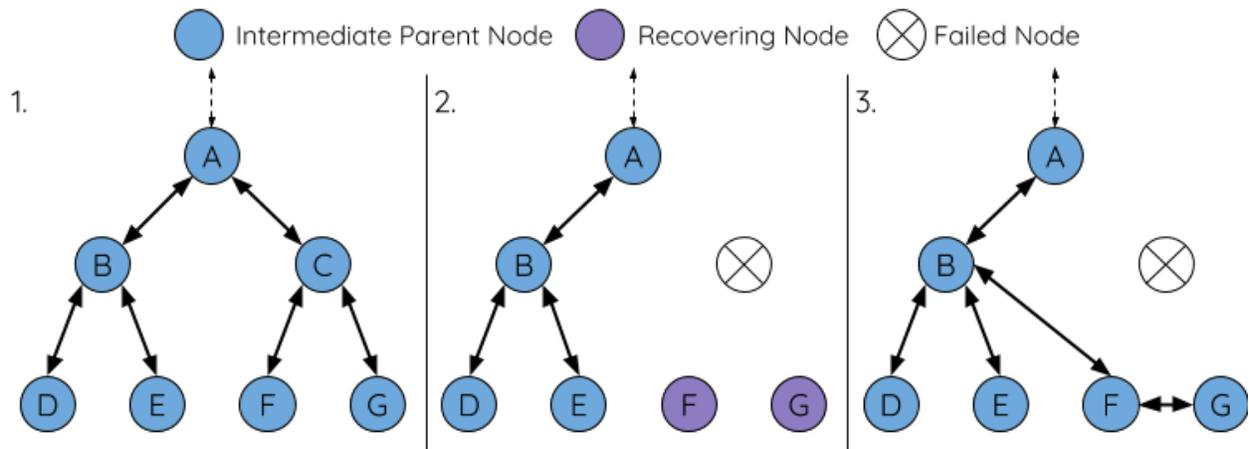
Fig. 55: Self Healing From Intermediate Parent Node Failure
