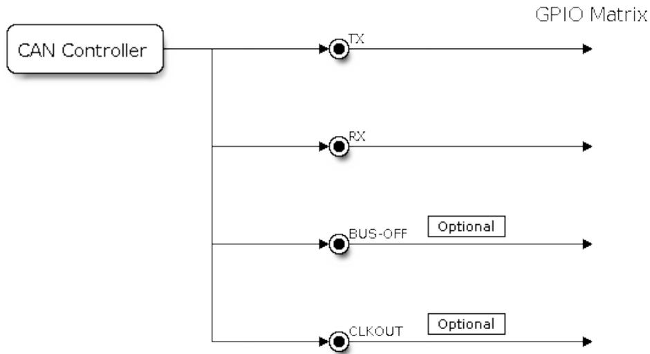
Fig. 7: Signal lines of the CAN controller
