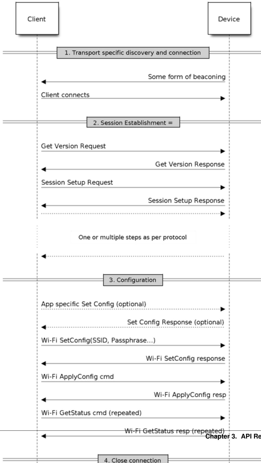
1. *Transport Security*: SoftAP provisioning may choose WPA2 protected security with unique per-device passphrase. Per-device unique passphrase can also act as a proof-of-possession. For BLE, “just-works” security can be used as a transport level security after understanding the level of security it provides.
