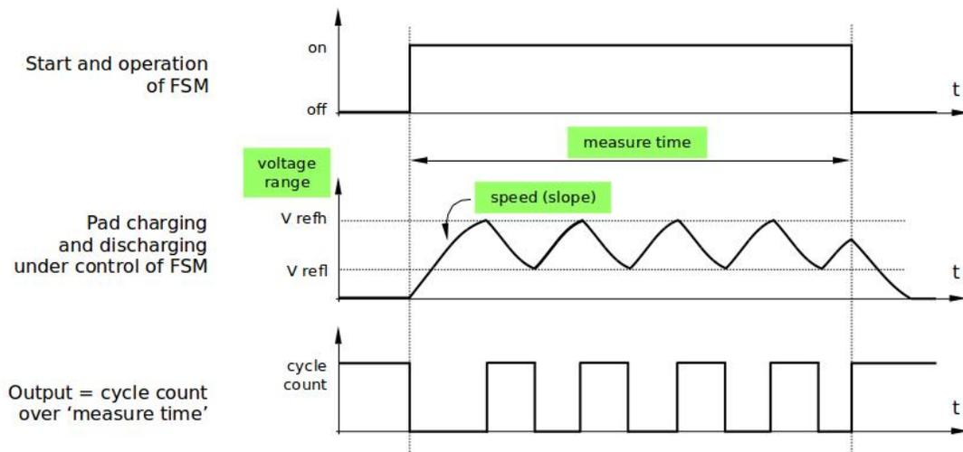
Fig. 22: Touch Pad - relationship between measurement parameters
