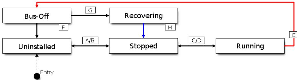
Fig. 11: State transition diagram of the CAN driver (see table below)
