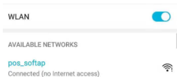
Fig. 1: Connection to the ESP32-C6 AP
