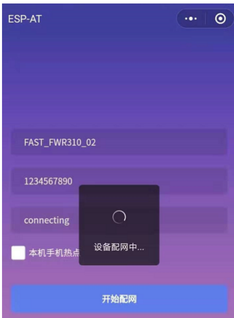
Fig. 16: Connection to the Router via the Applet
