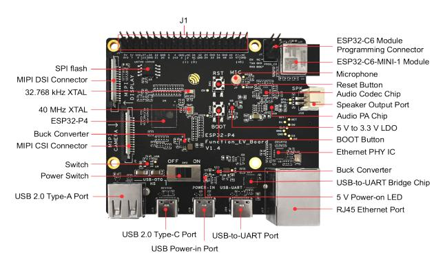
Fig. 7: ESP32-P4-Function-EV-Board - front (click to enlarge)
