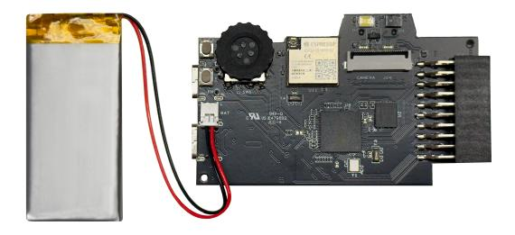
Fig. 8: Battery Connection (click to enlarge)
