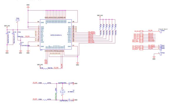
Fig. 17: ESP32-C6-MINI-1U Module Circuit (Click to Enlarge)
