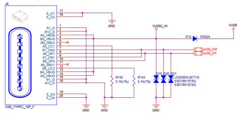
Fig. 10: USB 2.0 Device Port Circuit (Click to Enlarge)
