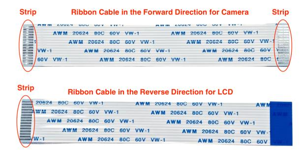
Fig. 9: Ribbon Cables in Forward and Reverse Directions
