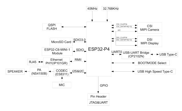
Fig. 10: ESP32-P4-Function-EV-Board v1.4 (click to enlarge)
