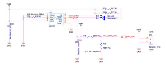
Fig. 13: Charging Circuit (Click to Enlarge)
