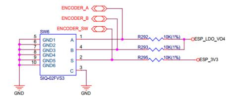
Fig. 16: Rotary Encoder Circuit (Click to Enlarge)
