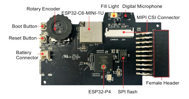
Fig. 5: ESP32-P4-EYE PCB Bottom View (click to enlarge)
