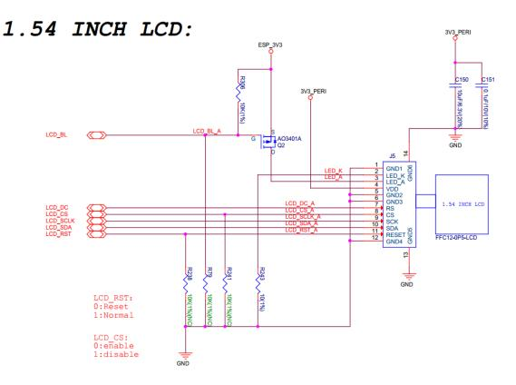
Fig. 11: LCD Circuit (Click to Enlarge)
