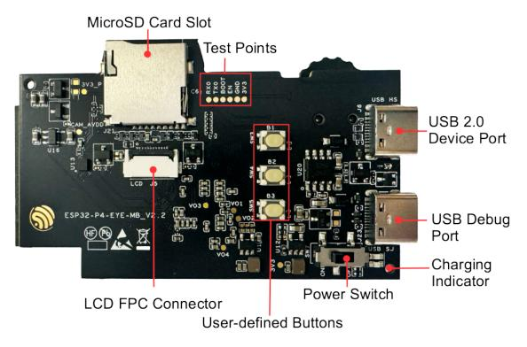
Fig. 3: ESP32-P4-EYE PCB Top View (click to enlarge)
