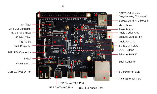
$Fig.\ 2:\ ESP32-P4-Function-EV-Board\ -\ front\ (click\ to\ enlarge)$
