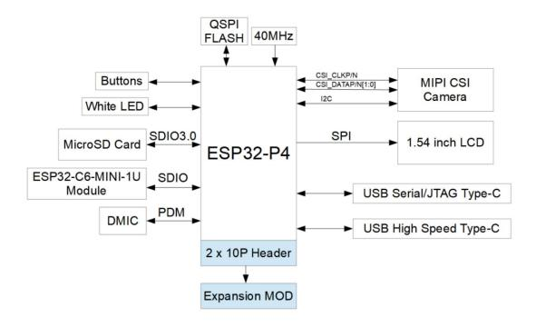
Fig. 7: ESP32-P4-EYE Functional Block Diagram (click to enlarge)
