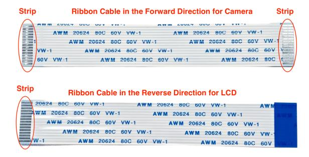
Fig. 4: Ribbon Cables in Forward and Reverse Directions
