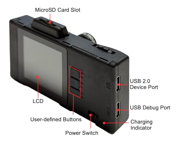
Fig. 4: ESP32-P4-EYE Front View (click to enlarge)
