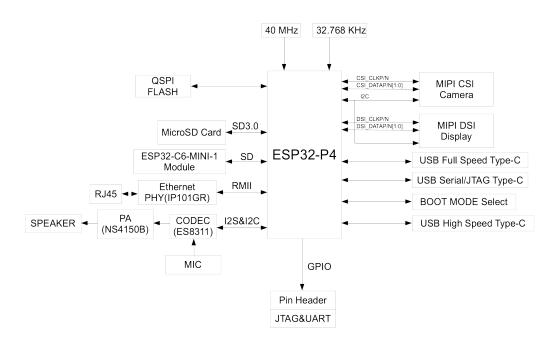
Fig. 5: ESP32-P4-Function-EV-Board Block Diagram (click to enlarge)
