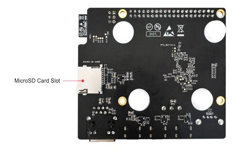
Fig. 8: ESP32-P4-Function-EV-Board - back (click to enlarge)
