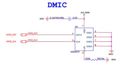
Fig. 14: Microphone Circuit (Click to Enlarge)
