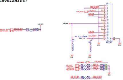
Fig. 15: Camera Circuit (Click to Enlarge)
