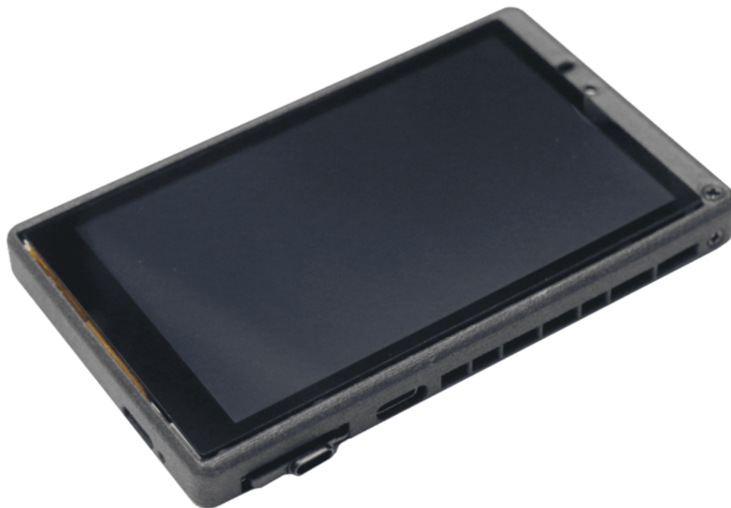
图 1: ESP32-S2-HMI-DevKit-1 (板载 ESP32-S2-WROVER 模组)
