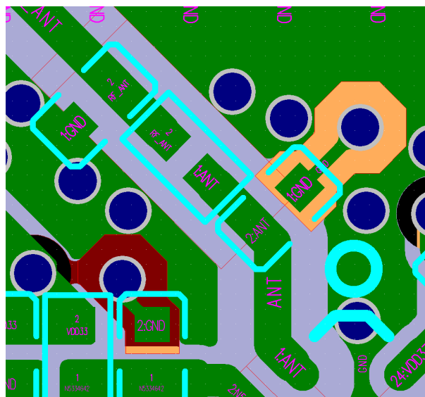
Fig. 10: ESP32-C2 Stub in a Four-layer PCB Design
