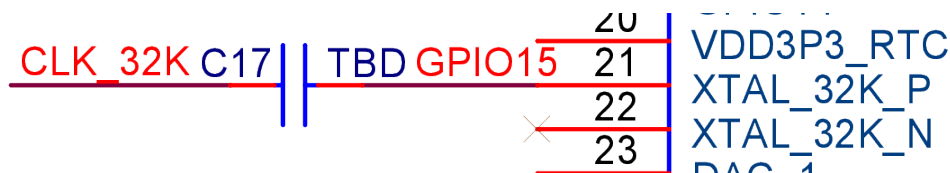
Fig. 9: ESP32-C3 Schematic for External Oscillator
