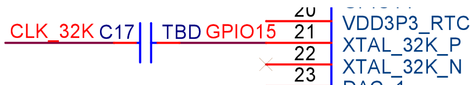
Fig. 9: ESP32-C3 Schematic for External Oscillator
