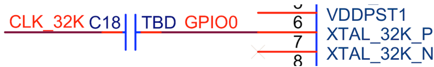
Fig. 9: ESP32-C6 Schematic for External Oscillator
