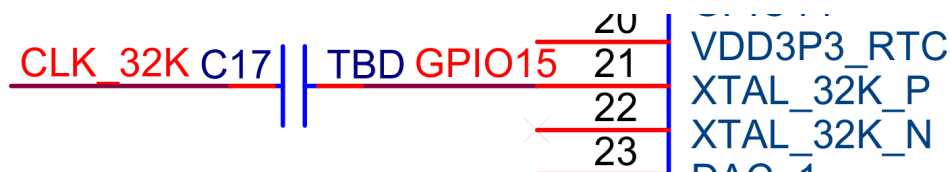
Fig. 9: ESP32-S2 Schematic for External Oscillator
