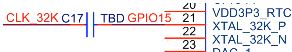
Fig. 9: ESP32-S3 Schematic for External Oscillator
