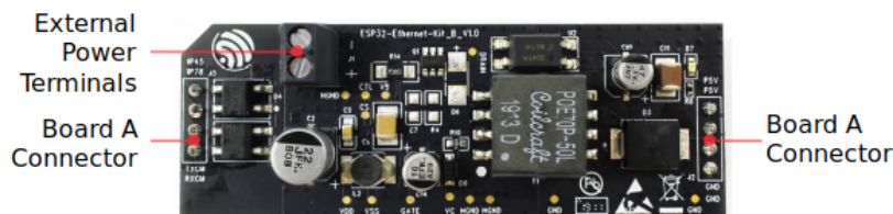
Fig. 30: ESP32-Ethernet-Kit - PoE board (B) layout (click to enlarge)
