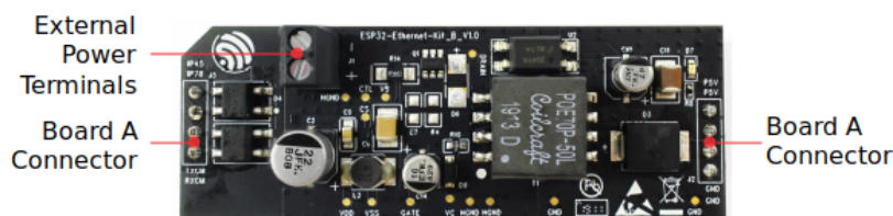
Fig. 35: ESP32-Ethernet-Kit - PoE board (B) layout (click to enlarge)
