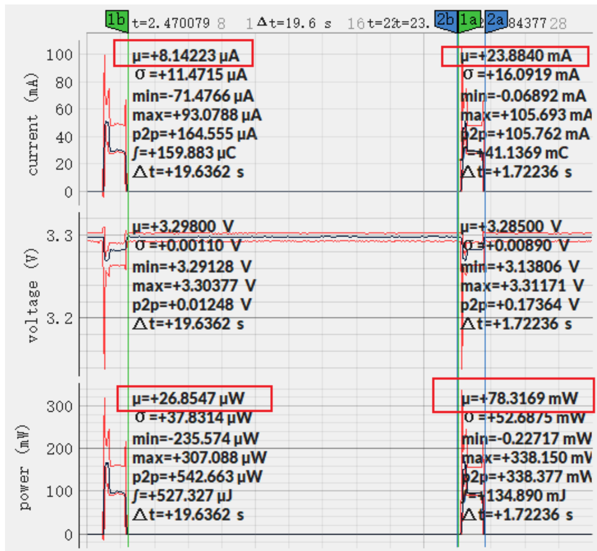
Fig. 43: Current Waveform of ESP32-S3-WROOM-1 (click to enlarge)
