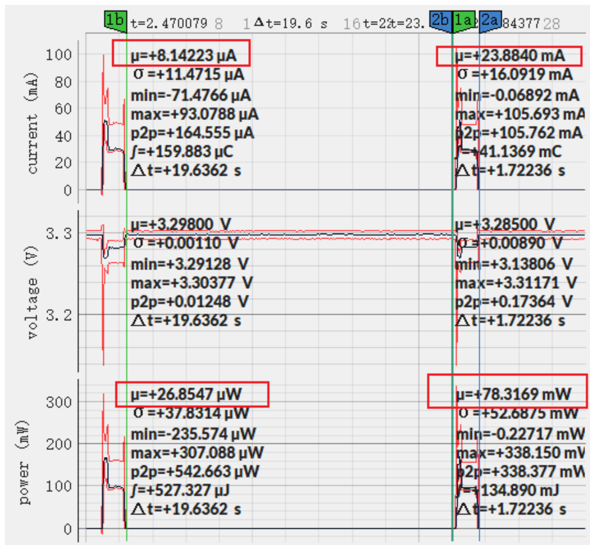
Fig. 7: Current Waveform of ESP32-S3-WROOM-1 (click to enlarge)
