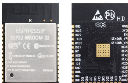
Fig. 1: ESP32-WROOM-32 module (front and back)
