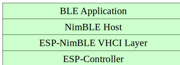
Fig. 1: ESP NimBLE Stack
