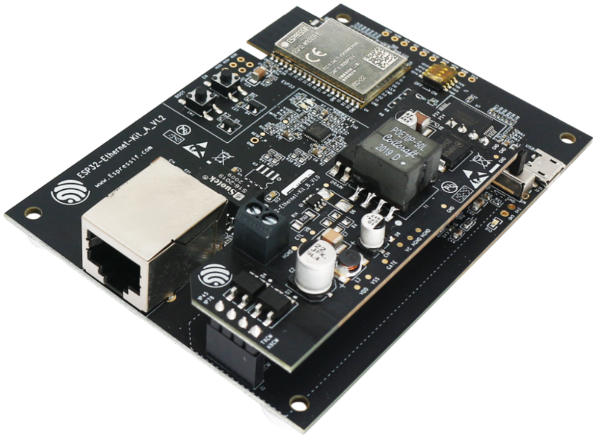
Fig. 21: ESP32-Ethernet-Kit V1.2 Overview (click to enlarge)
