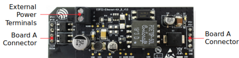
Fig. 25: ESP32-Ethernet-Kit - PoE board (B) layout (click to enlarge)
