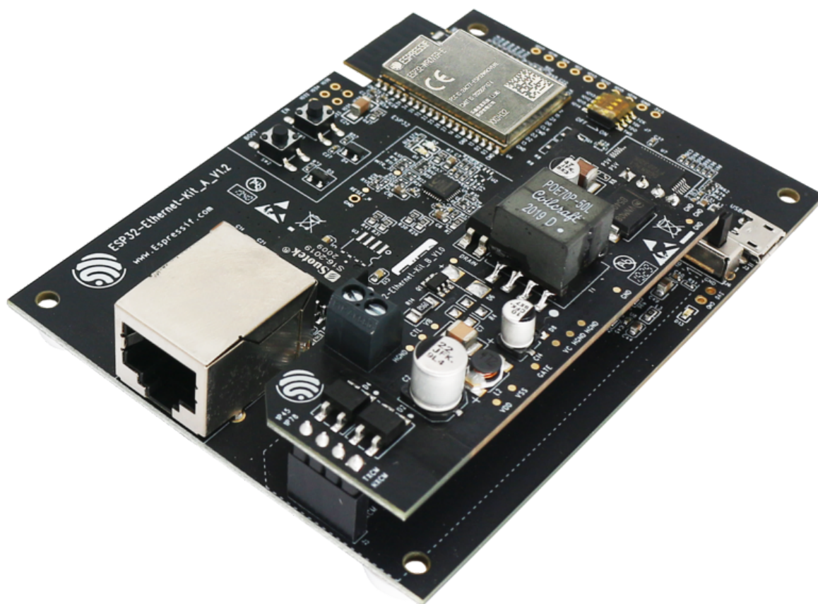
Fig. 21: ESP32-Ethernet-Kit V1.2 Overview (click to enlarge)
