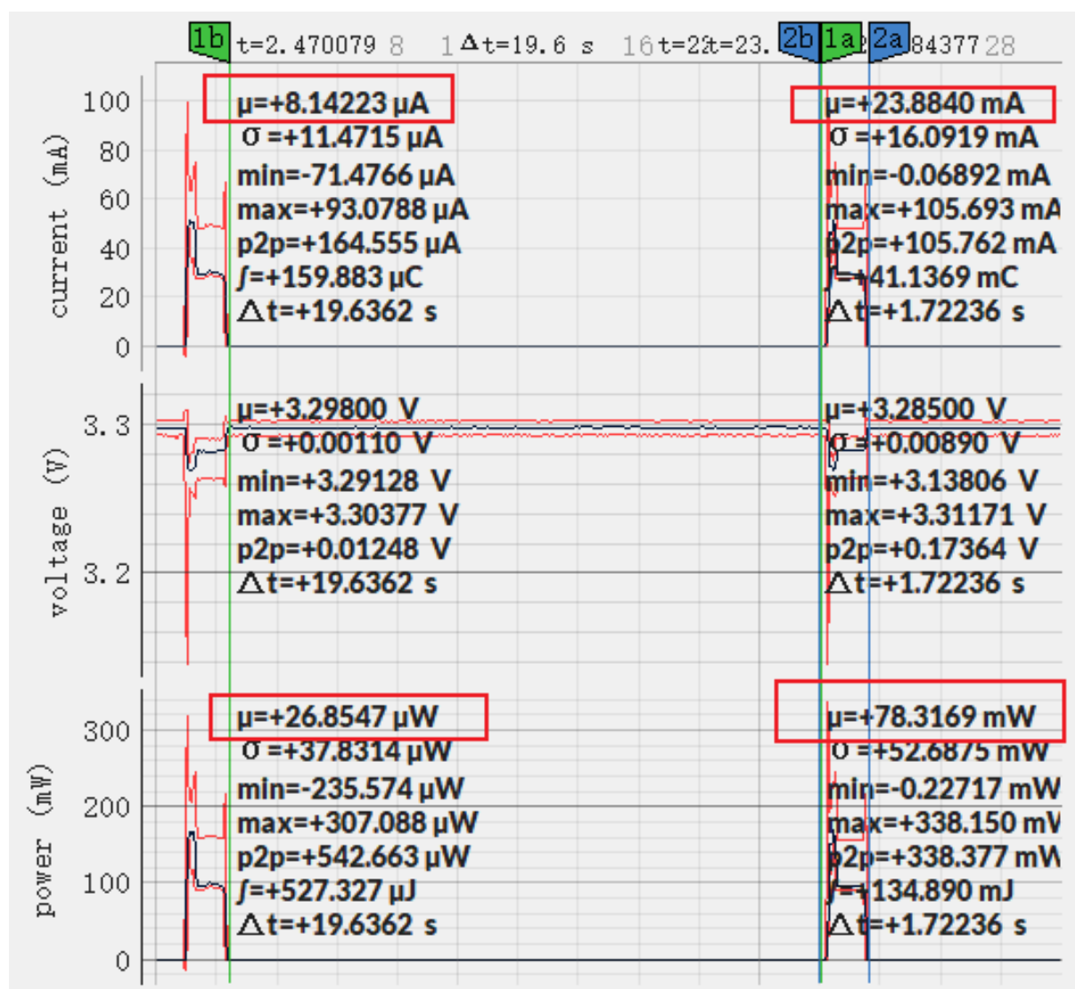
Fig. 11: Current Waveform of ESP32-S3-WROOM-1 (click to enlarge)
