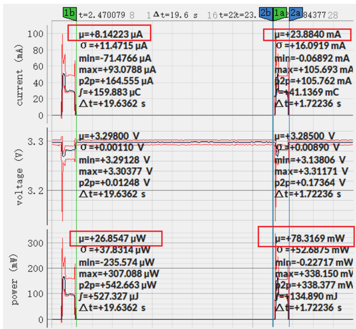
Fig. 43: Current Waveform of ESP32-S3-WROOM-1 (click to enlarge)
