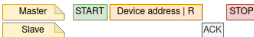
图 13: I2C master probe
