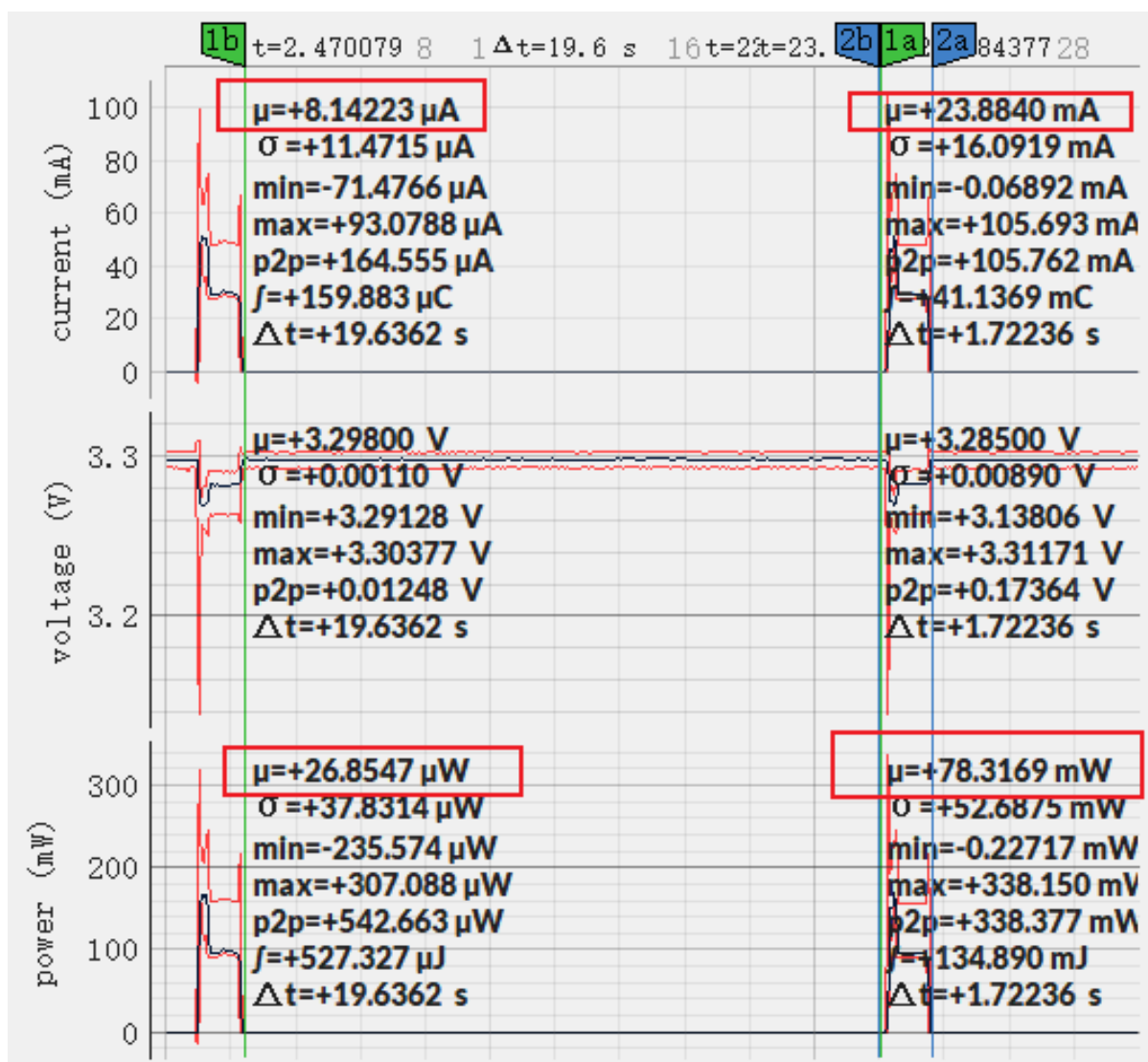
图 7: Current Waveform of ESP32-S3-WROOM-1 (click to enlarge)
