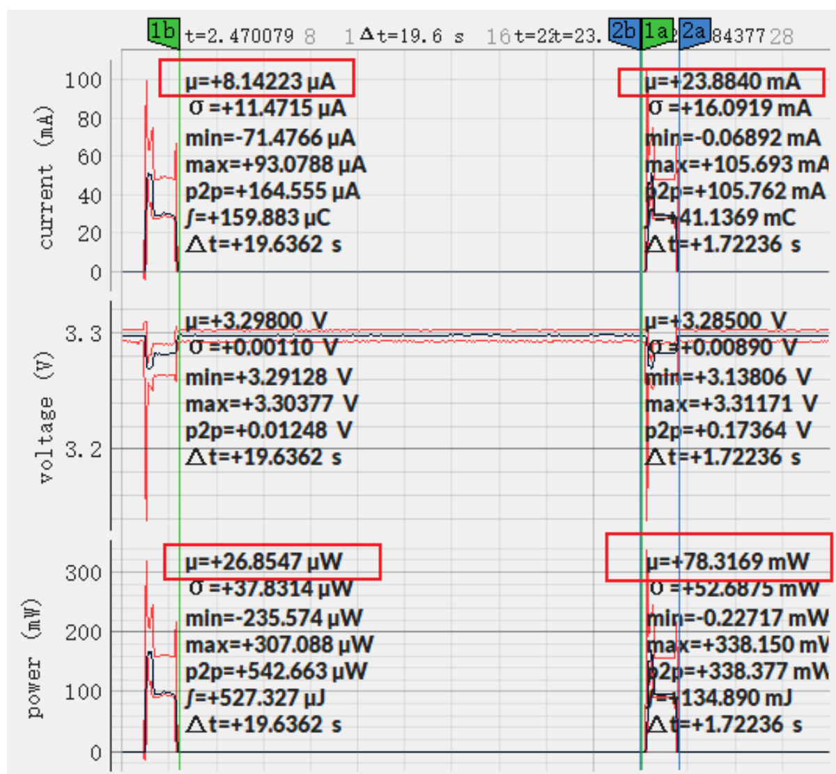
图 31: Current Waveform of ESP32-S3-WROOM-1 (click to enlarge)
