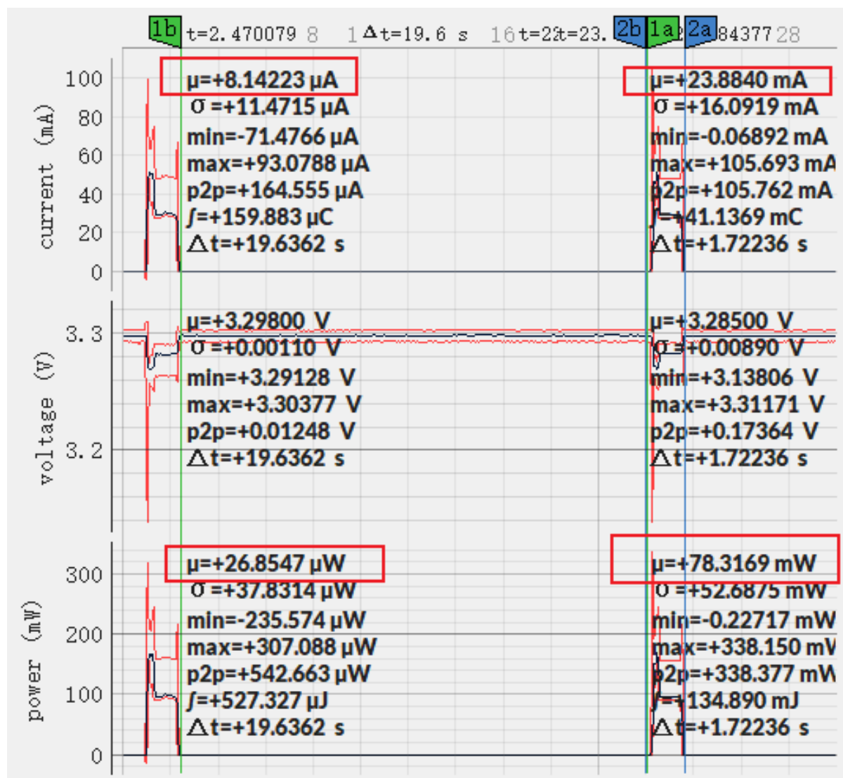
图 11: Current Waveform of ESP32-S3-WROOM-1 (click to enlarge)
