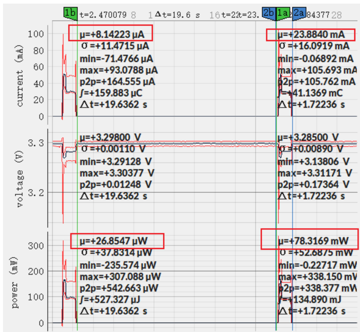
图 11: Current Waveform of ESP32-S3-WROOM-1 (click to enlarge)
