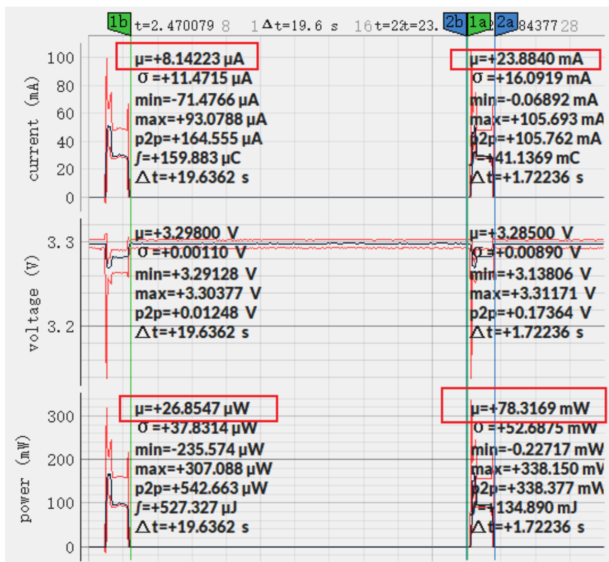
图 11: Current Waveform of ESP32-S3-WROOM-1 (click to enlarge)
