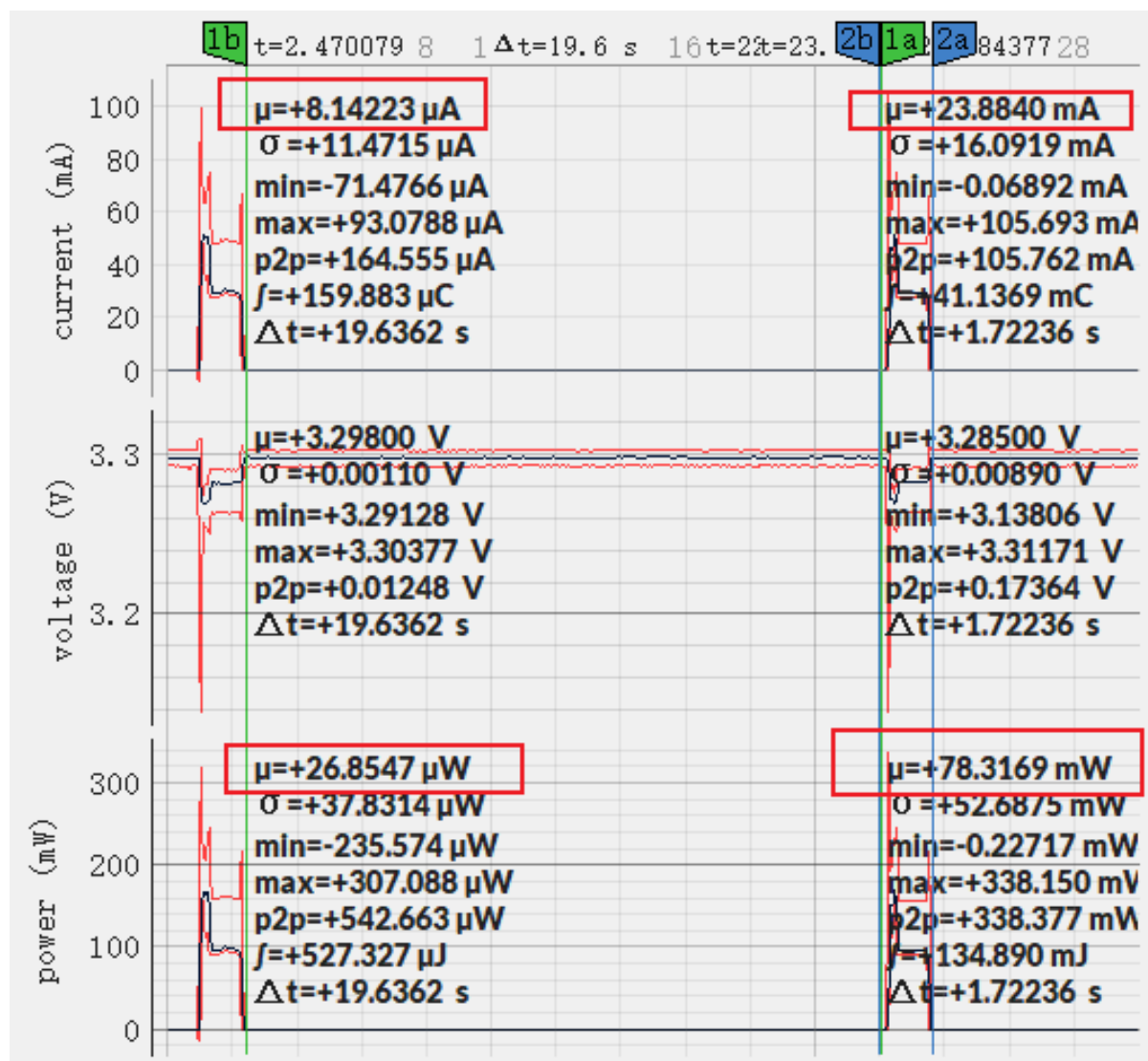
图 7: Current Waveform of ESP32-S3-WROOM-1 (click to enlarge)
