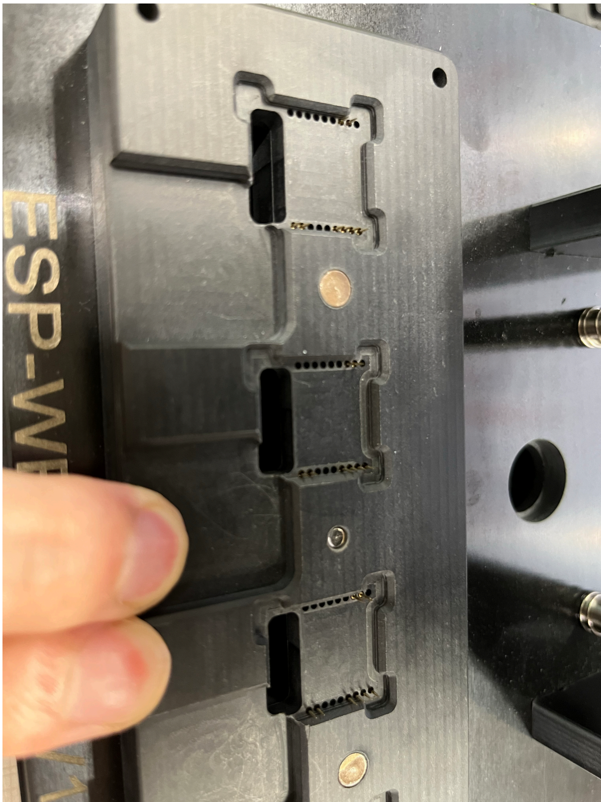
Fig. 85: The Metal Probes (the handle is pressed)
