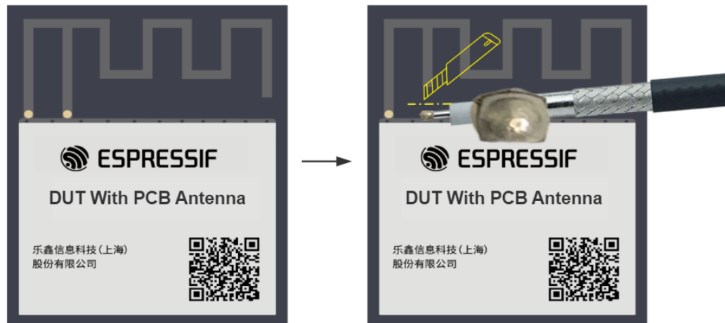
Fig. 25: Soldering RF Connection Cable to Module with Onboard PCB Antenna
