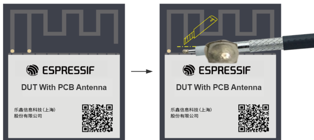
Fig. 40: Soldering RF Connection Cable to Module with Onboard PCB Antenna
