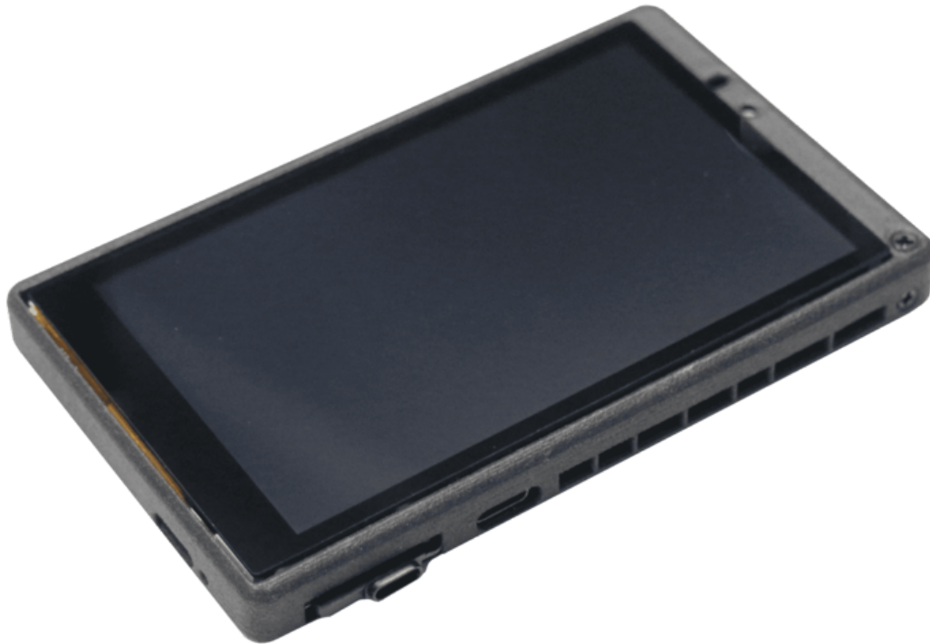
Fig. 5: ESP32-S2-HMI-DevKit-1 with ESP32-S2-WROVER module
