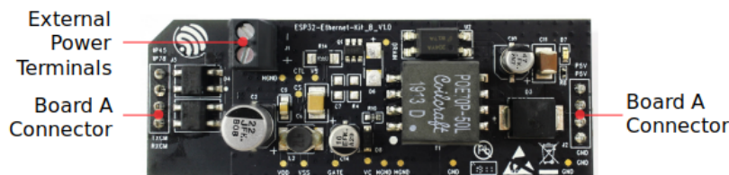
Fig. 30: ESP32-Ethernet-Kit - PoE board (B) layout (click to enlarge)
