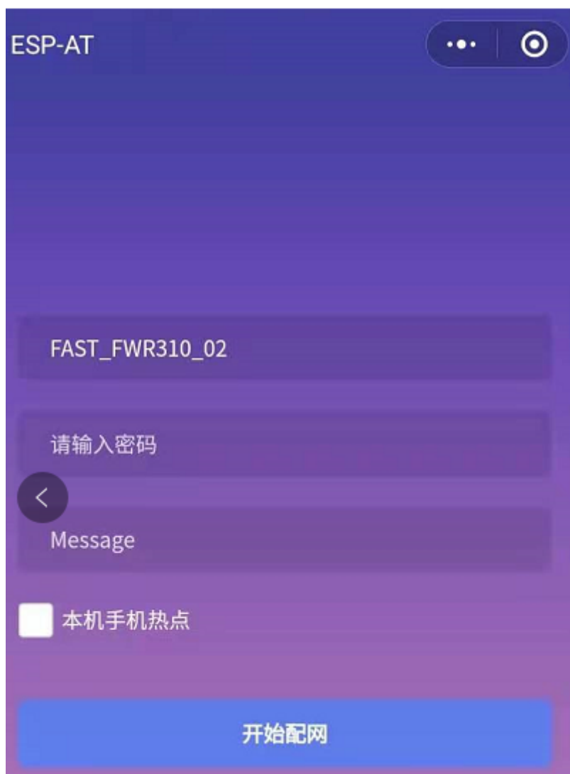
Fig. 14: Getting Router Information
